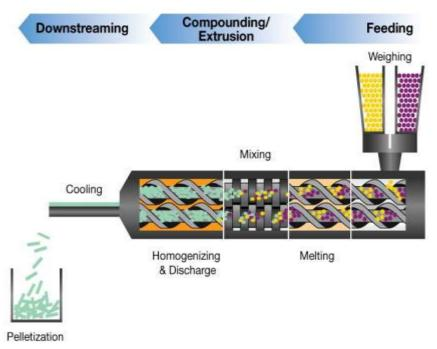
The Melt Extrusion Process
